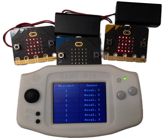
Figure 1: Two battery powered micro:bits log accelerometer data and send it over radio to a micro:bit with a display shield, which saves it to flash storage and displays it in a tabular format.
